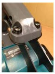
**33.** Attach the other handle bracket the same way but don't tighten that side yet.
