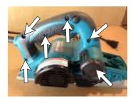
**3.** Remove the 5 handle screws and pull off vacuum port plug. One side of the handle will pull off, the other is snapped into the housing at rear. Pry the snap lock with a flat screw driver (photo) while tapping the side of the handle off. Doesn't matter if you break it, just don't tear up the housing getting this off.
