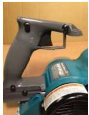
**31.** Fit the other half of the handle in place and make sure the wires are still in place. Secure the handle halves with 3 self-tapping black screws and tighten. Then install the screw opposite the one from step 30, use the same washer sequence but do not tighten yet.
