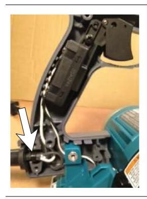
30. Position the switch and dress the wires <u>EXACTLY</u> as shown. There are slots in the handle that separate the cord and motor wires. Screw the switch down. Make sure the cable tie (arrow) is positioned correct and that the rubber cord boot is in the handle groove. The handle half may wobble and some of the wires can pop out of place, just push them back in position and try and stabilize everything. Use a flat screwdriver to jam them in place if needed.
