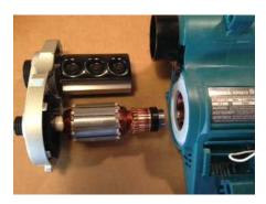
**19.** Put the cover plate with the cutter and armature partially into the housing and turn it over.
