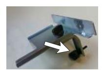
**5.** Your Makita came with a fence like this. Remove the thumbscrew shown and put aside. This is the longer of the two screws and may have an O-ring holding it, just cut it off.
