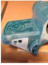
**16.** These 2 raised features at the front of the housing have to go so that they won't interfere with holding the planer with the new knob. Grind / cut down, sand smooth.
