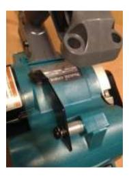
**32.** Get the right side handle bracket from the kit and attach the threaded standoff (shorter one) using the same screw and washers as the handle. Tighten the screw and push the standoff in the hole of the housing lug.
