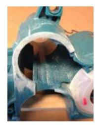
**13.** Fit the adapter back into the housing. The housing must be trimmed along this inside corner at the arrow flush with adapter; rough cut then sand smooth.
