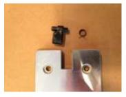
**6.** Remove the 4 screws attaching the base and remove. Remove the little kick-stand and spring at the rear and discard. Keep the base plate and screws.
