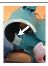
**14.** There is a raised feature inside the port, measure in from the edge 5/8" (16mm) and mark. Grind this down so that the opening is circular. There's another one directly above, grind that one down also. No need to be pretty, leave rough.
