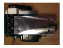
**22.** Take the 2 wires from the motor out of the plastic guide on top. Re-route them through the hole below as shown. Pull them tight. Then replace the motor cover (2 screws) and the base plate (4 screws).
