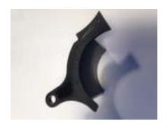
**12.** The next cut is right at this inside corner, tape 1/16" away as before and rough cut. Sand / file this cut until flush and the previous 2 also
