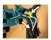
**4.** Remove the wires from the switch and remove cord clamp. There should be nothing left attached to the planer just the white & black wires coming out of the motor. Keep the cord with the rubber boot, nothing else will be reused here.
