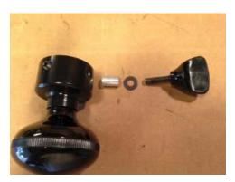
**25.** Assemble the upper knob as shown, tighten the big screw. Then install the thumbscrew (step 5) using the spacer and flat washer. Do not tighten yet, check that it doesn't protrude into the big hole of the collar. If so, back it out. Same with both of the setscrews.
