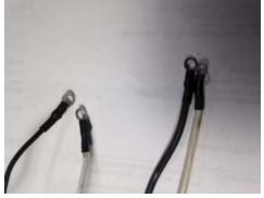
27. Now is the time to shorten your cord if running up a vac hose. Crimp the terminals on the wires from the cord and the motor. If you don't have the proper crimp tool, solder them. Put the cable tie on the cord (arrow), pull tight and trim. Put the heat-shrink tubing over the terminals as shown. Shrink down with a heat gun / lighter / matches / candle or whatever your habits acquire. Just don't burn the house down.
